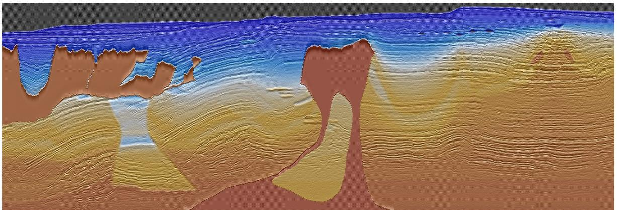
Figure 2: velocity model interleaved with the reflectivity. The vertical scale has been exaggerated twice. We can see the complexity of the signal and notice that velocity and reflectivity have similar trends in some areas only.
