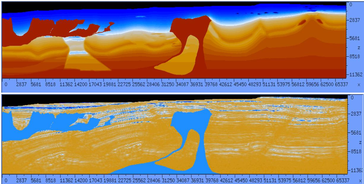
Figure 1: (top) velocity model and (bottom) density model used to generate the dataset.
